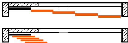
4 MOVING DOOR SLIDING SYSTEM SWSF 051-4
