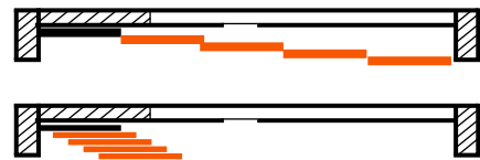
4 MOVING DOOR SLIDING SYSTEM SWSF 022-4
